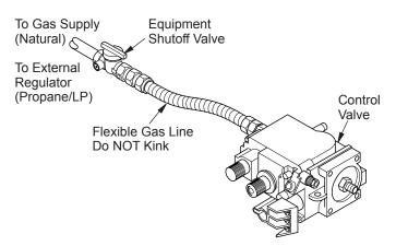
Figure 32 - Connecting Flexible Gas Line to Control Valve
